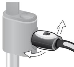
3. Pull the milk frother (6) to open it. The appliance heats up. Hot water runs out of the milk frother outlet (6) for about 40 seconds.
