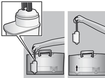
**Note:** You can use the filter indicator to mark the month in which you inserted the filter. You can also mark the month in which you will need to replace the filter next (at the latest after two months).
